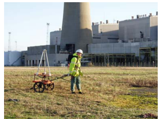
Geophysical surveying at the E.ON Isle of Grain Power Station
