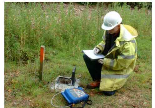
Environmental monitoring of ground gases for land quality assessment
