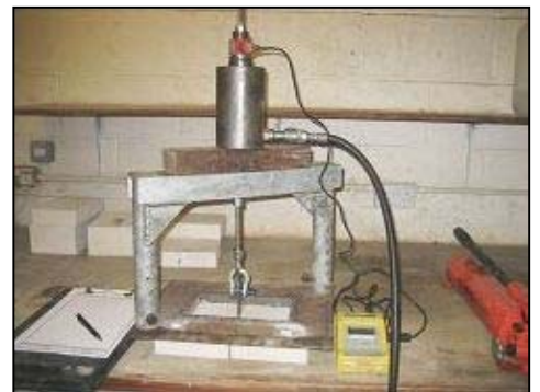
Laboratory tests on stone dowel fixings
