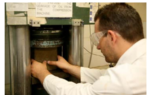
Compressive strength testing
