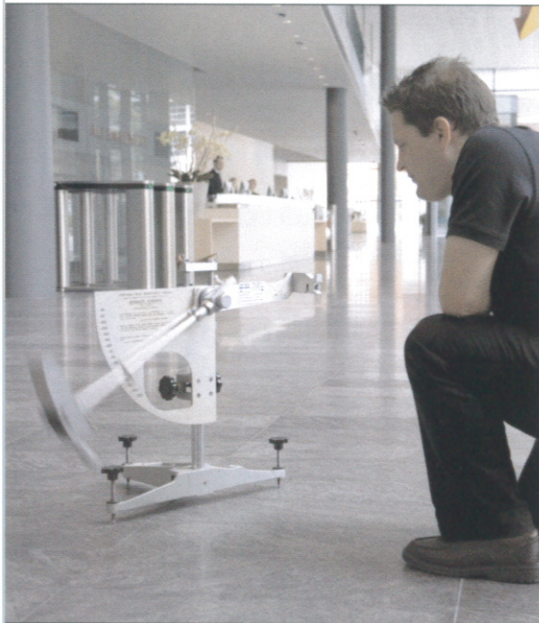
The pendulum swinging during the test. The instrument measures the distance the pendulum swings after contact with the surface being tested.
