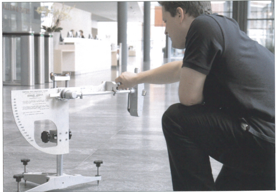
Setting up the weighted pendulum to test the slip resistance of a floor.
